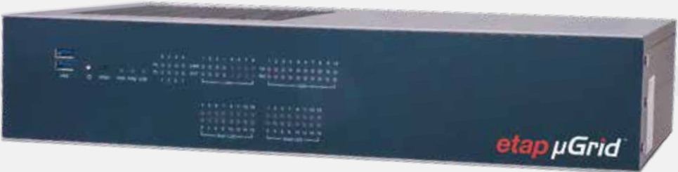
Controller logic is validated using ETAP Software-in-the-Loop technology
